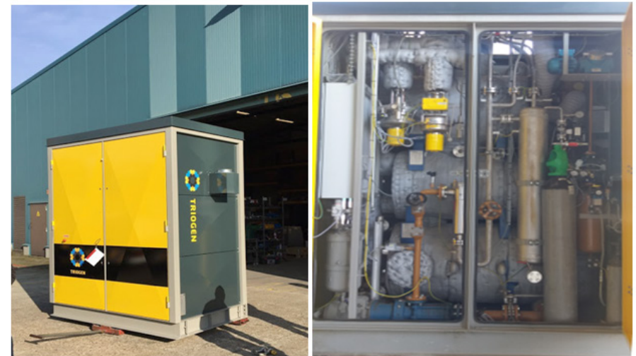
(a) (b) Figure 1. (a) Triogen E-box (b) Process inside E-box
